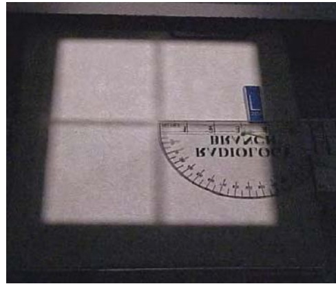
Figure 4-40. Measuring eight-inch restricted CF so LM is within four inches from the center.
